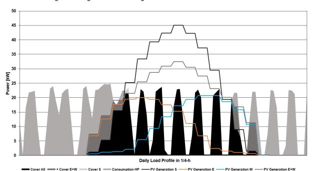
Figure 1: Comparison of a PV system with a south and east-west orientation for the power supply of a high-temperature heat pump
